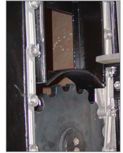
DuraMax cast stainless steel chain and urethane sprockets newly installed in 2005 (above); and same today (below) looking hardly any different.
